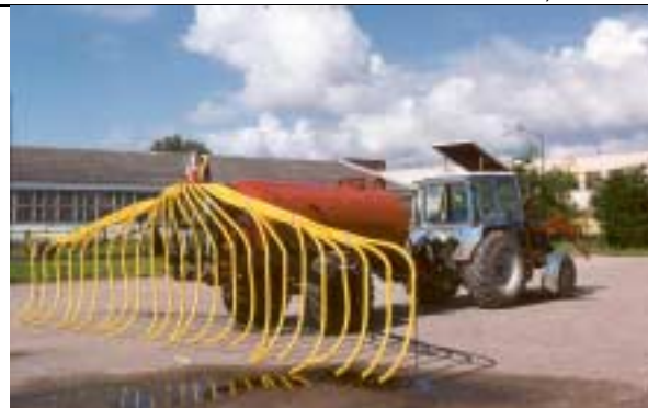
Fig. 3. Hose slurry and liquid manure spreader attached to slurry tank MZT-6
