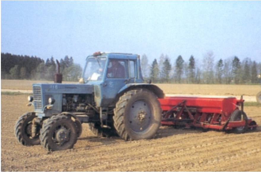
Fig. 3.7. Sugar beet seedier TUME KOMBI – 7, which places fertiliser locally.
